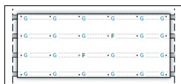
FIG. G - Horizontal installation on horizontal profiles. When there is an even number of fastener columns as shown, the Fixed points should be diagonal from one another to provide equal weight distribution.
