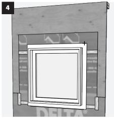
window in accordance with manufacturer's specifications. Generally, the gap between window and rough opening should be around 1/2" (12 mm).
